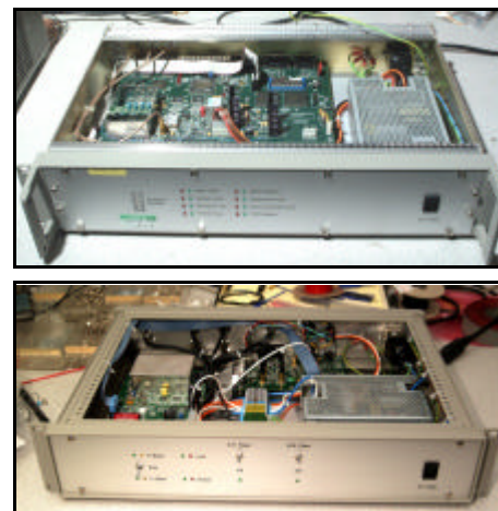
Fig 5: One of the new Programmable Receivers (top) and an associated IF Multiplexer (bottom).
